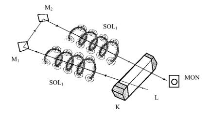
If one does not make use of a device different from a Kerr's cell, the luminous beam should be polarized since the beginning, making it for instance reflect on the surface of a semi-silvered glass plate. Furthermore, because of a possible new polarization assumed by the luminous beam at the interior of the solenoid, it would be better to find in any case an alternative to the Kerr's cell. The required effects could
